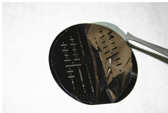
Fig. 1. The parylene shadow mask being peeled off a wafer after fabrication.
